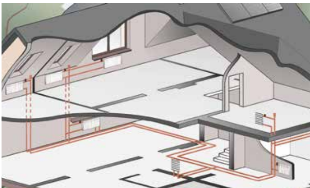
“Vertical” system in a heating installation
