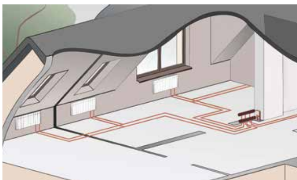
Manifold – tee system in a heating installation
